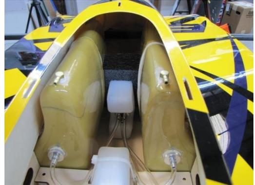
NOTE: We use Safety Wire inside the tanks to secure fittings and we use Spring Clamps on the outside.
