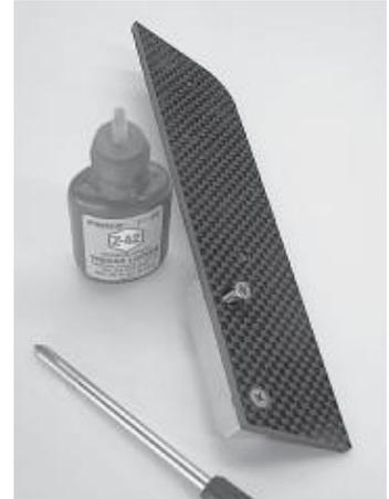
NOTE: Topside of plates have larger 6-32 screw countersinks and bevel on outside edge. Z-42 Thread Locker is for metal-to-metal threads only.
